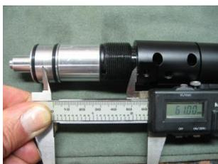
Place a piece of masking tape on the centerline of the cylinder along the bottom of the cylinder. Draw a straight line on the tape along the centerline, and transfer the dimension of the breather hole to the cylinder.
