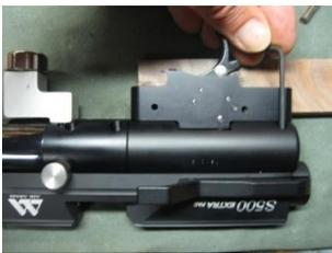
The Breech and Barrel assembly can now be lifted from the rest of the rifle body. Be careful not to lose the white plastic seal washer, it can fall off easily.
