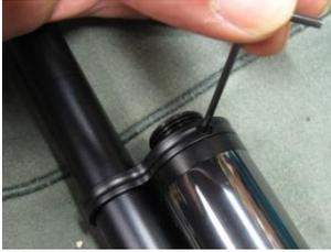
Remove the two screws from the end of the Striker Body. (Note this is a S500 FAC assembly and does not have anti-tamper devices plugging the screw holes. If your model is not FAC, the plugs will need to be removed.) Remove the four screws from the Valve Body in front of the trigger. These screws will be easier to remove if the trigger guard is removed first.
