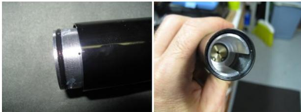
Regulator installed and valve body fully threaded into place. Use the hose clamps, rubber strips, and protective rag in the bench vise to get a good grip on the cylinder for tightening. Be sure to align the witness marks made earlier during final tightening of the valve body. This ensures the proper torque on the connection.
