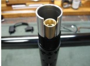
Coat the inside of the cylinder and the outer surface of the regulator with silicone grease. Gently press the regulator into the cylinder with your thumb until it passes the inside threads of the cylinder. Make sure the breath hole of the regulator body is facing upwards to the breech when the tube is screwed on. Then position the spacer in front of the regulator and press the two together further into the cylinder until the threads are exposed enough to thread the valve body into place.
