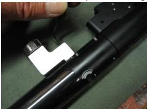
Before removing the cylinder, make a small mark across both the cylinder end and the valve body. This will give a reference point to tighten the cylinder to at re-assembly. Again, a very tightly torqued connection.
