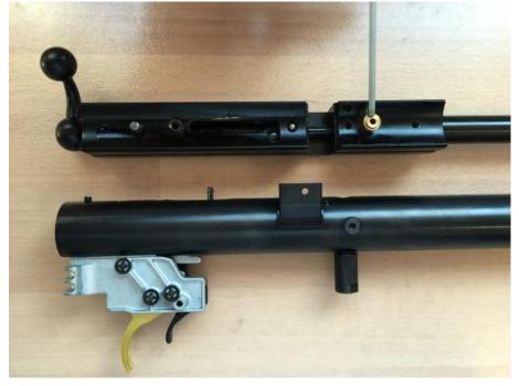
Unscrew the triggergroup and after you have removed it you see an allen bolt inside the hammer, when you loosen it you can take out the hammer latch pin.
