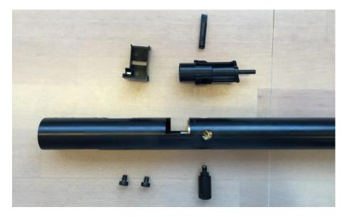
With an allen key or a piece of wood you can easily unscrew the fillcap from the pressure tube.
