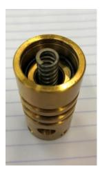
First check the inner walls of the valvehouse with the biggest diameter if it is free of scratches. If not please polish them properly.
