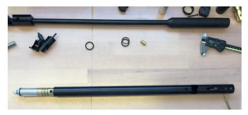
Place the transfer port what you have opened up in diameter to 4-4,2 mm back in it's place. Place all three screws back in their place and turn them in. **Tighten them AFTER you have assembled the breech in the right position.**
