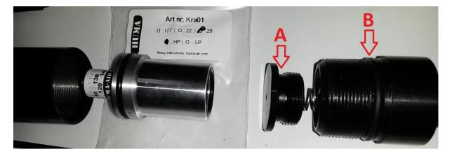
Unscrew the valvehouse cap and place the small o-ring what came with the regulator on the cap "A" Then grease the o-ring seating on the valvehouse a bit for smooth fitting.
