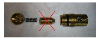
Replace the original BSA house for the regulator and screw it on the valve house.
