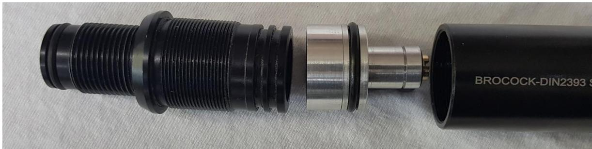
Make the the treads of the tube and valvehouse clean of grease and screw it back into the pressure tube. Tighten it by hand, and after you have tighten it unscrew the valvehouse for about a quarter of a turn leaving a tiny gap between tube and adapter. This will help your regulator to breath free.
