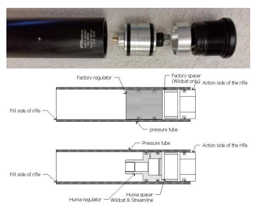
Check if the regulator is fully clean and free of dirt. If not, clean it and apply some silicone grease on the walls of the pressure tube. Then slide the new regulator into the pressure tube, facing the label side to the barrel end.
