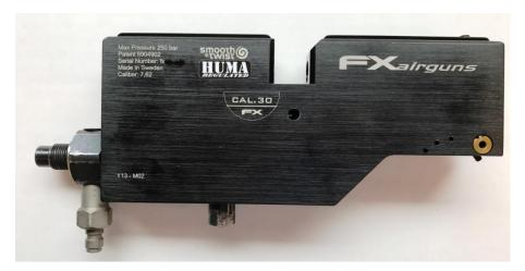
Please check if the adapter does not touches the setscrew when it is screwed in again by measuring the length. (If it does, the reg needs to be pushed into the rifle some more OR open up the hole in the bottle adapter for about 2-3 mm in length and 8 mm diameter, but this is very unlikely)
